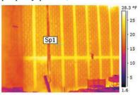
of discontinuity or voids that could compromise the structural integrity of the wall system.
